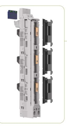
The feeder meter (TSA) is assembled in an upper case on top of the fuse switch. This case includes three protection fuses.
