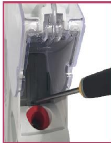
Window opening for access to the busbar
